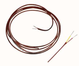
Thermocouple wire is a specialized type of wire used to measure temperature. It's made of two different metals joined at one end, creating a junction. When the junction is exposed to different temperatures, a voltage is generated that can be measured and converted into a temperature reading.
