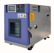
Constant Temperature Humidity Test Chamber Temperature range -20°C→+150°C (adjustable) Introduction.
