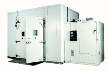
A Temperature and Humidity Control Chamber, often called an environmental chamber, is a specialized device used to simulate specific climatic conditions. It is essential for testing and evaluating how products, materials, or systems perform under varying temperature and humidity levels. These chambers are widely used in industries such as HVAC, automotive, electronics, aerospace, and pharmaceuticals.
